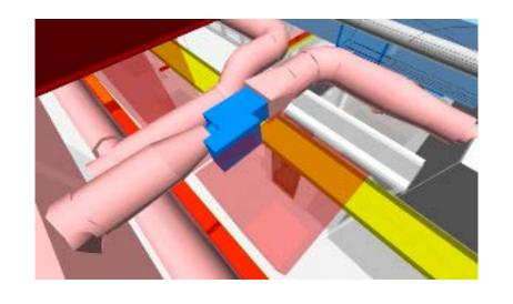
• VAV Clearance must be identified and observed.
